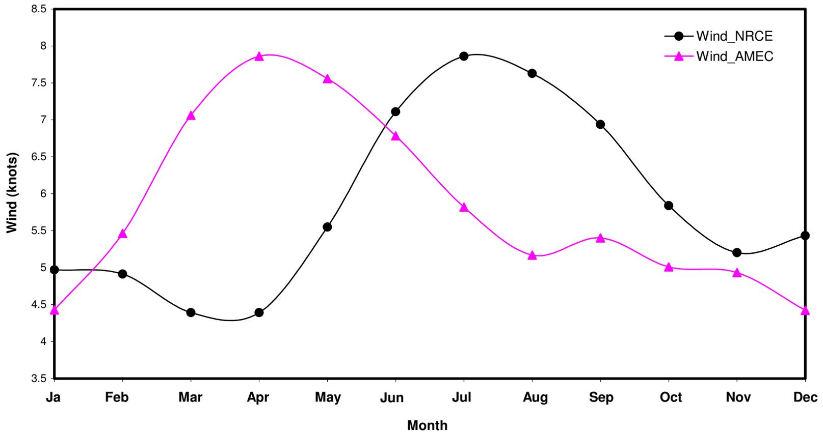
Figure 7: Comparison of the NRCE reported and AMEC calculated monthly pattern of the wind data for the Gallup municipal airport weather station
