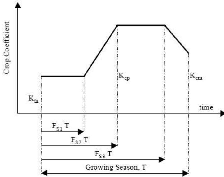
Figure 12. Pattern of the basal crop coefficient ( $K_{cb}$ ) during a growing season (Source: NRCE, 2008).
